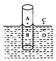
Suppose that capillary tube is dipped into a liquid, which wets the capillary tube. The shape of the water inside the capillary tube is concave.
